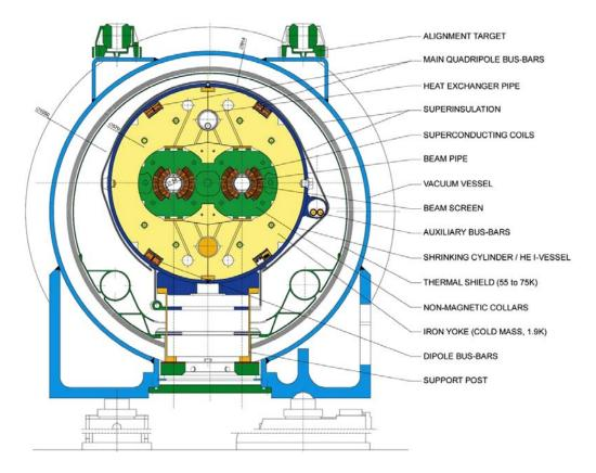
Figure 3.3: Cross-section of cryodipole (lengths in mm).
