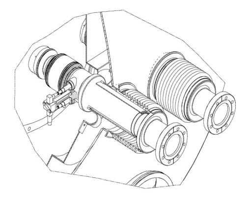
Figure 5.5: Details of a cold-to-warm transition.
