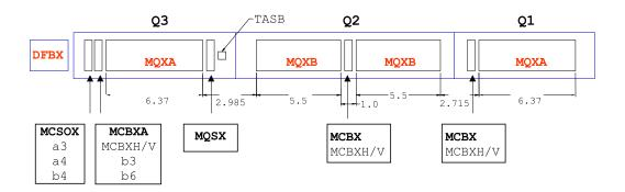
Figure 3.16: Schematic layout of the low- $\beta$  triplet (distances in m).
