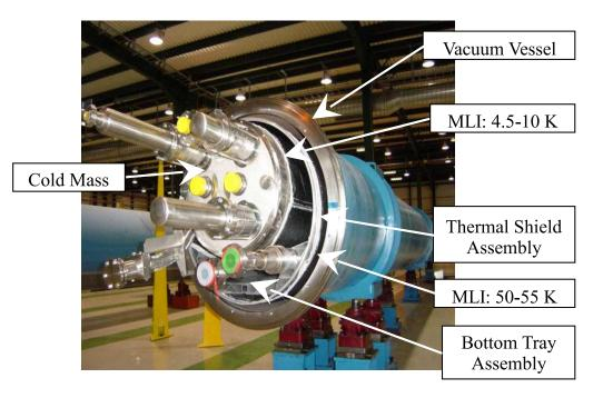
Figure 3.5: LHC dipole cryomagnet assembly.
