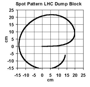
Figure 10.5: Beam spot figure on absorber block.
