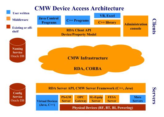
Figure 9.4: The Device Access Model.
