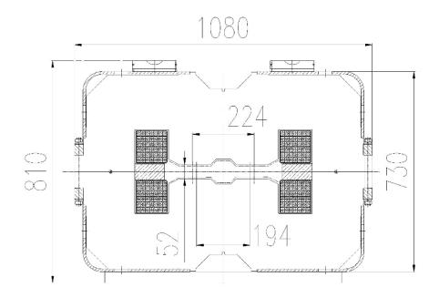
Figure 3.14: Cross-section of the normal conducting separation dipole MBW (dimensions in mm).
