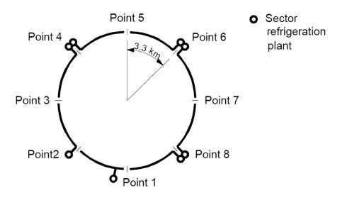
Figure 7.2: General layout of the cryogenic system.
