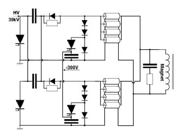
Figure 10.4: Dual branch generator circuit layout.
