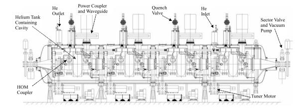
Figure 4.1: Four-cavity cryomodule.
