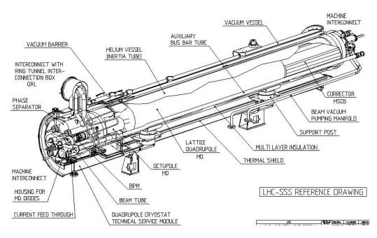
Figure 3.6: Short straight section with jumper.
