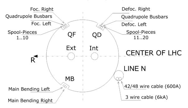
Figure 6.3: Cross-section of LHC arc cryo-assembly with bus-bars.
