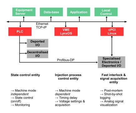
Figure 11.8: MKI control system architecture.
