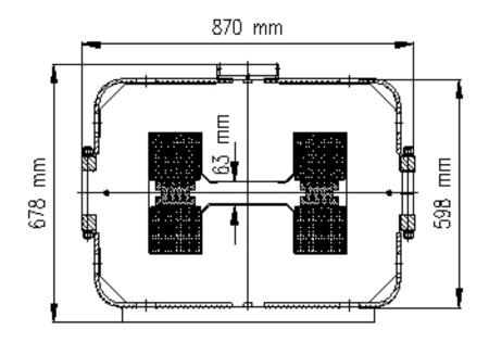
Figure 3.15: Cross-section of the normal conducting separator dipole magnet MBXW.
