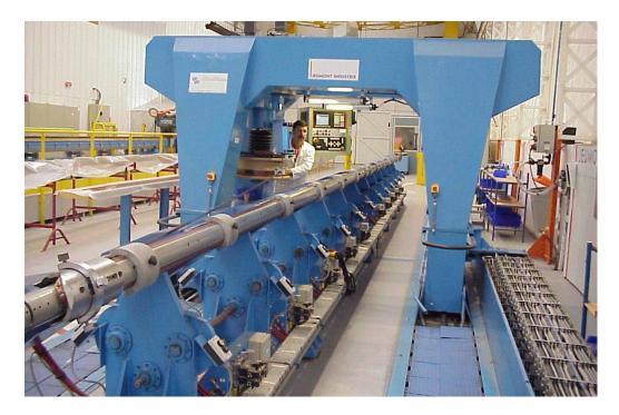
Figure 3.4: A winding machine for the superconducting coils.
