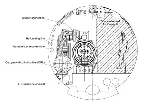
Figure 7.1: Transverse cross-section of the LHC tunnel.
