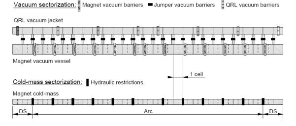
Figure 7.6: Cold-mass and cryogenic vacuum sub-sectorisation.
