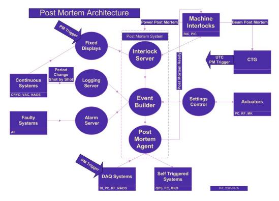
Figure 9.8: The LHC Post Mortem Architecture.
