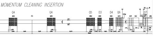
Figure 2.7: Schematic layout of the matching section on the right side of IR3 (distances in m).
