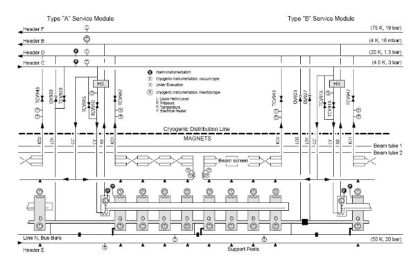
Figure 7.5: Thermodynamic cryogenic flow scheme and instrumentation of an LHC lattice cell.
