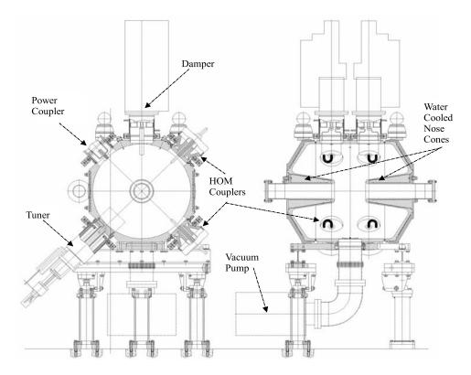
Figure 4.3: ACN 200 MHz cavity mounted on its support.
