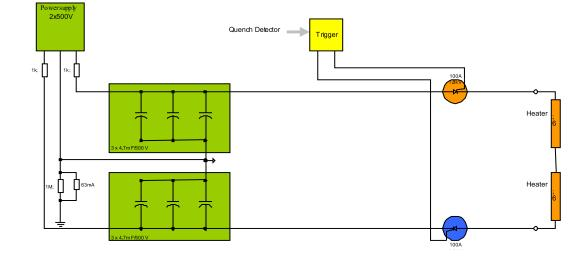
Figure 6.7: Quench heater power supply functional diagram.
