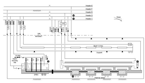
Figure 7.8: Cryogenic flow scheme and instrumentation of an inner triplet cell.
