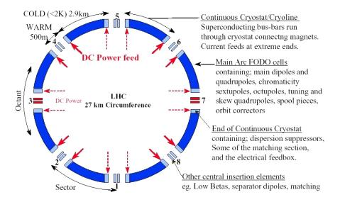
Figure 6.2: Powering of the eight arc cryostats.
