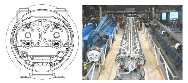
**Figure 3.13**: Cross-section of the MBRS dipole (left) and assembly of the MBRS cold masses at BNL (right).
