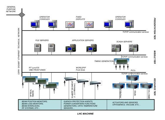
Figure 9.1: Control system architecture.
