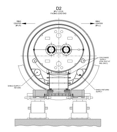
Figure 3.12: Cross section of the MBRC (D2) cryodipole at a support post location.
