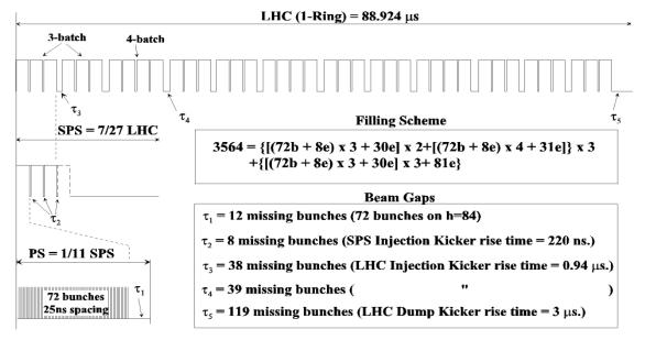
**Figure 12.2**: Proton bunches in the PS, SPS and one LHC ring. Note the partial filling of the SPS (3/11 or 4/11) and the voids due to kicker rise-time. One LHC ring is filled in  $\sim 3 \text{ min.}$
