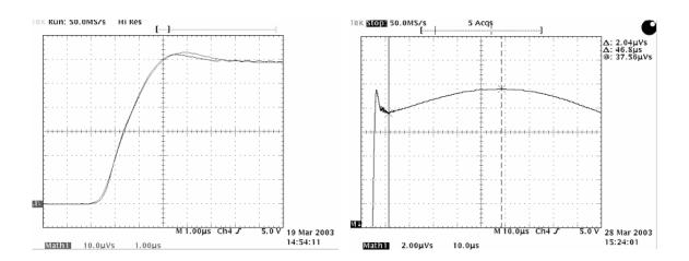
**Figure 10.2**: Start of MKD magnet current pulse at 450 GeV and 7 TeV with overshoots of 7.5% and 5.2% respectively (left); MKD magnet current pulse over 100  $\mu$ s at 7 TeV with flat top overshoot of 5.6% (right).
