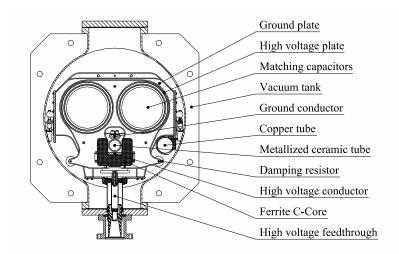
Figure 11.6: MKI magnet cross section.
