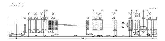
Figure 2.4: Schematic layout of the right side of IR1 (distances in m).
