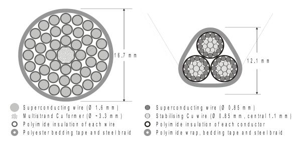
Figure 6.6: Cross sections of the  $42 \times 600$  A cable (left) and the  $3 \times 6$  kA cable (right).
