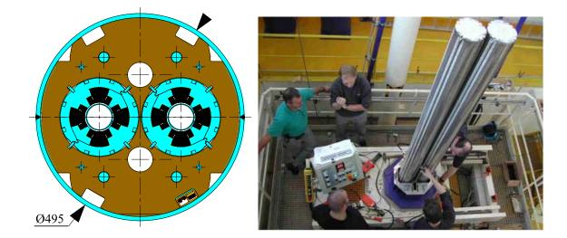
**Figure 3.9**: Cross-section of MQY quadrupole (left) and assembly of the magnet (right) (dimensions in mm).
