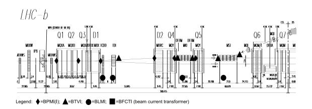
**Figure 11.9**: Schematic view of injection related instrumentation (case of injection near Point 8) (distances in mm).
