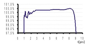
Figure 11.7: MKI prototype current pulse shape (top part of scale).
