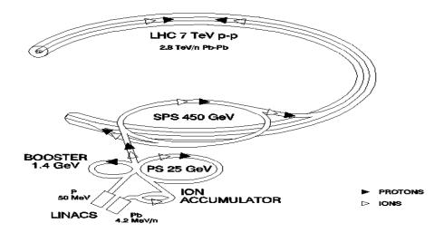
Figure 12.1: The LHC injector complex.
