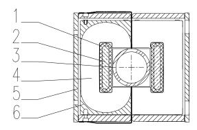
Figure 10.3: Cross-section of the MKD magnet.
