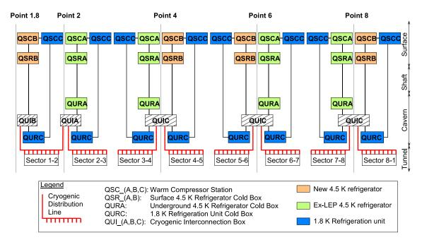
Figure 7.3: General architecture of the cryogenic system.
