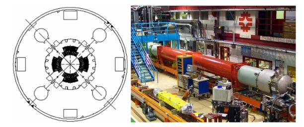
**Figure 3.18**: Cross-section of the MQXB low- $\beta$  quadrupole (left) and Q2 quadrupole on test in FNAL (right).
