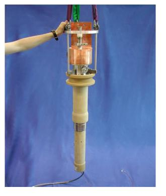
Figure 6.5: 13 kA CERN prototype HTS current lead.
