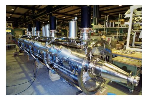
Figure 4.2: Four-cavity module during assembly.
